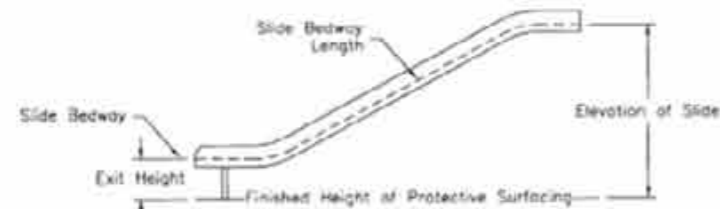
Note 1—If elevation is \geq 48 in. (1220 mm) exit height shall be between 7 in. (180 mm) and 15 in. (380 mm). If elevation is \geq 48 in. (1220 mm) exit height shall be 11 in. (280 mm) maximum. Reference Section 8.3.11.1. Note 2—Slide bedway length, for structural integrity purposes only, is denoted by the dashed line. Reference Section 10.4.2.2. FIG. A1.21 Height of Slide Exit Region and Slide Bedway Length Reference Section 8.3.11.1
